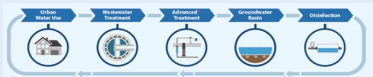
FIGURE 47 Schematic of groundwater augmentation process
