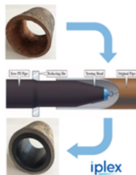
FIGURE 1 DIE REDUCTION LINING PROCESS
