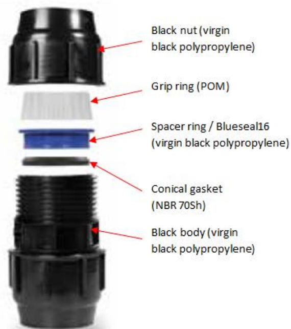
FIGURE 1: EXPLODED VIEW OF SAB BLUESEAL SEALING SYSTEM
