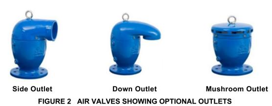
The air valves, suitable for water applications in pump stations and pipelines, evacuate air during pipeline filling, allow release of air pockets from pressurized pipes and enable large volumes of air intake in the event of network draining.
