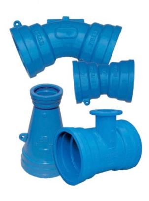
The TYTON® socket profile provides the flexibility of using TYTON gaskets for ductile iron OD compatible pipes, PLASTYT gaskets for series 1 PVC pipes or TYTON-LOK® gaskets for restrained joints. Joints can be deflected and permits axial movement to compensate for thermal expansion and contraction.
