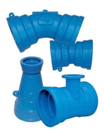
The TYTON® sacket profile provides the flexibility of using TYTON gaskets for ductile iron OD compatible pipes, PLASTYT gaskets for series 1 PVC pipes or TYTON-LOK® gaskets for restrained joints. Joints can be deflected and permits axial movement to compensate for thermal expansion and contraction.
